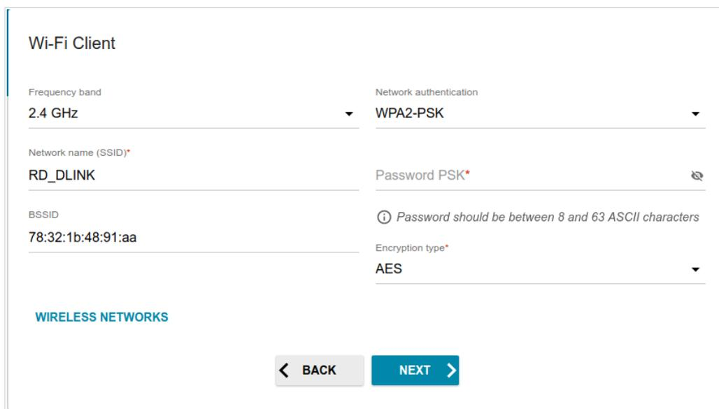
Figure 39. The page for configuring the Wi-Fi client.
