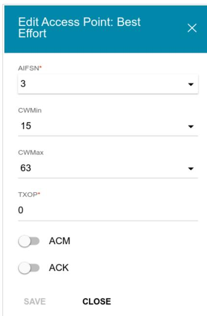
Figure 97. The window for changing parameters of the WMM function.
