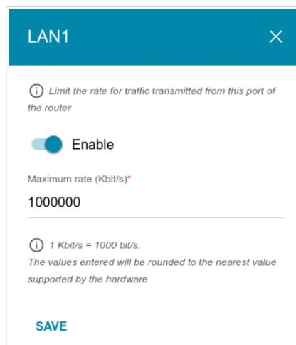
Figure 114. The window for setting up rate limit.
