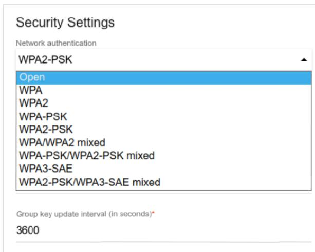
Figure 90. Network authentication types supported by the router.
