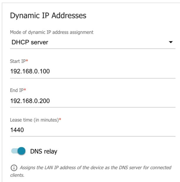
Figure 80. Configuring the local interface. The IPv4 tab. The Dynamic IP Addresses section.
