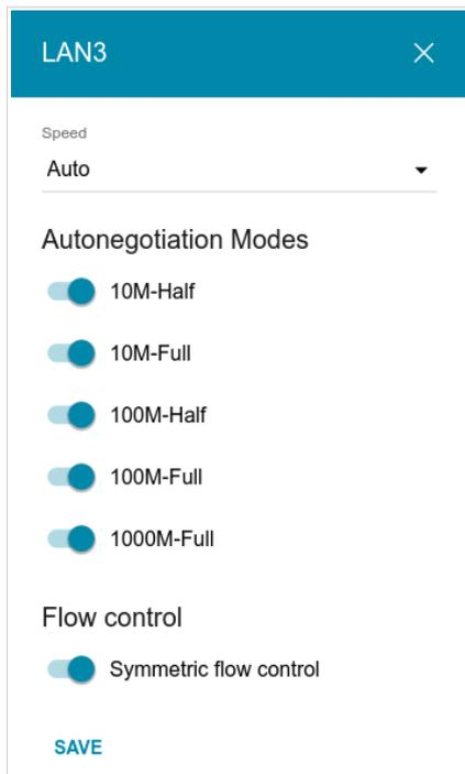
Figure 112. The window for changing the settings of the router's port.
