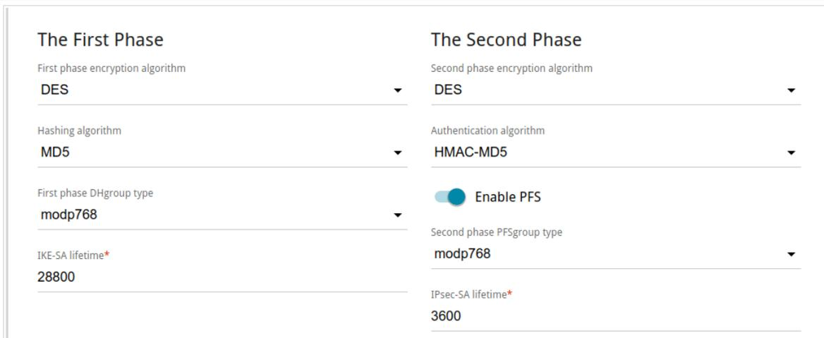
Figure 129. The page for adding an IPsec tunnel. **The First Phase / The Second Phase** sections.
