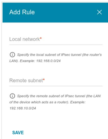
Figure 130. The page for adding an IPsec tunnel. The window for adding a tunneled network.
