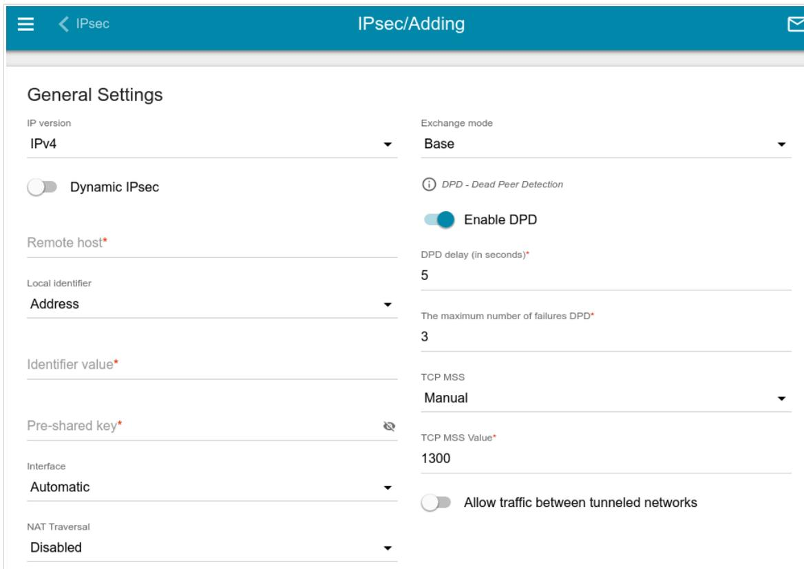
Figure 128. The page for adding an IPsec tunnel. The **General Settings** section.
