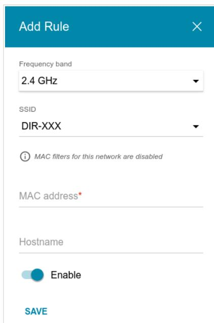
Figure 103. The window for adding a rule for the MAC filter.
